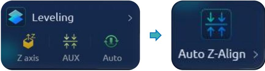
1 Click the “Leveling” on the main interface, the machine will auto home first. After the machine stops, click “Auto Z-axis Alignment”, and the whole X-axis beam of the machine will ascend to the top and then descend to zero again.
